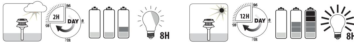
**GB** Note that the light brightness shall dim automatically, depending on the day's charge of the battery. This guarantees 8 hours of light output.
