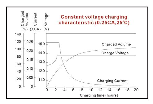
Note: it is necessary to ensure that the voltage is correctly set. A charging voltage set too high will increase the corrosion of the positive plates and shorten battery life. A charging voltage set too low will lead to sulphating of the plates causing loss of capacity and ultimately shortening the life of the battery.
