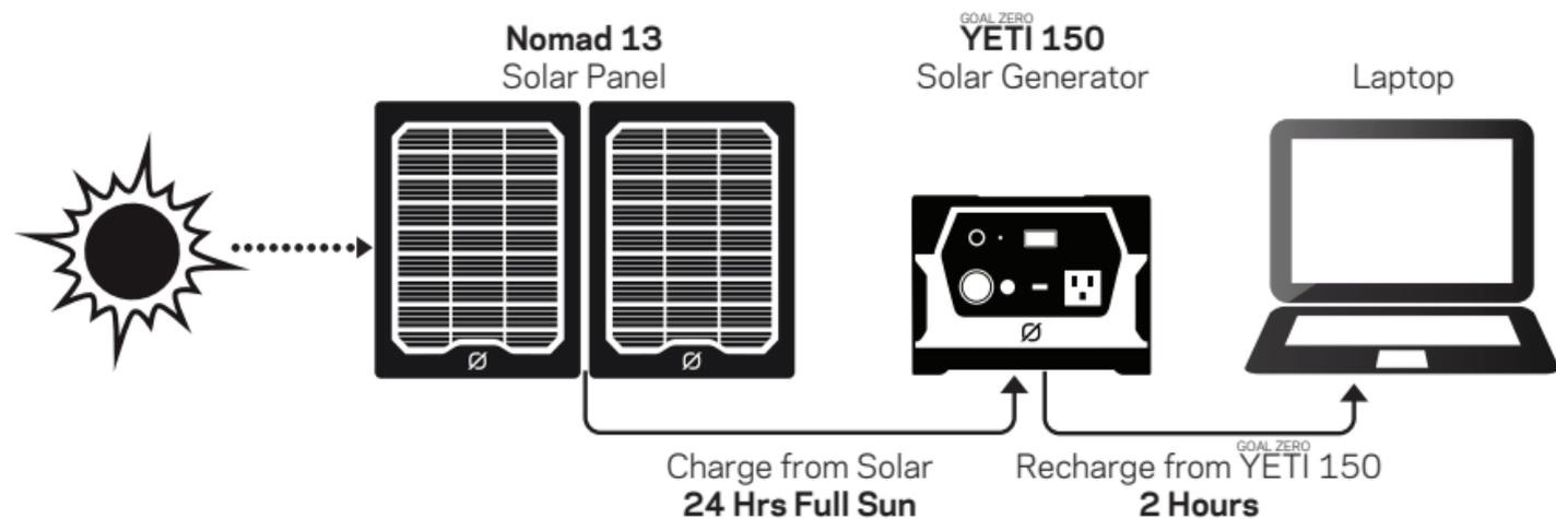
**Note:** Solar charging times depend on weather conditions. Charge YETI 150 from wall in 5 hours.
